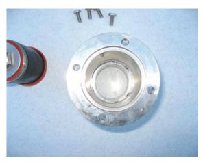
Just out of habit I like to draw a line as a point of reference with a permanent marker on the cover and flange of the RV body so that when we replace the cover, the sensing elbow stays
