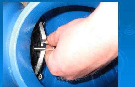
Once the retainer is removed the check module can be pulled straight out of the body.
