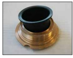
inside-out. At this point you can smooth out any wrinkles or bubbles and then slide the main-stem through the guide and into the diaphragm. Turn the assembly over onto the main-stem so that the diaphragm is pointing up. Push down
