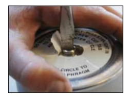
exposed. I try to only cut a couple of the tabs on the sticker so that hopefully I can replace this part of the sticker upon completion. Now take a slotted screwdriver and remove the screw while applying pressure with your other hand to control RV spring tension.
