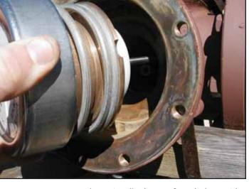
the outer diaphragm from being cut by this screw. To remove the module, grasp the outer edges of this (button) and pull it straight out of the body.
