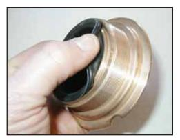
fingers and push the diaphragm back through the guide so that it's inverted or
