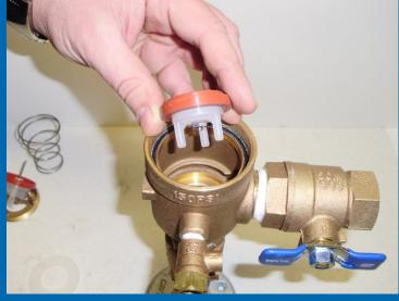
The disc is free once the screw and guide are removed.
