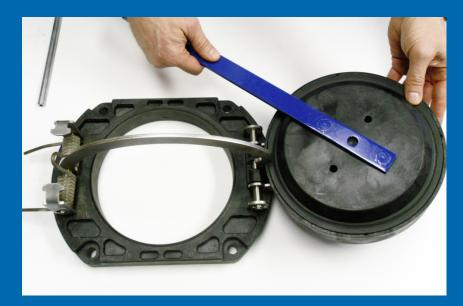
Once the disc retainer has been removed, the check disc is free.
