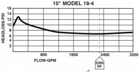
10" model 18-4" Flow curve generated by the Foundation for Cross-Connection Control and Hydraulic Research at the University of Southern California.
