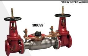
Series 3000SS Double Check Detector Assemblies are designed for use in accordance with water utility non-health hazard containment requirements. It is mandatory to prevent the reverse flow of fire protection system substances, i.e., glycerin wetting agents, stagnant water and water of non-potable quality from being pumped or siphoned into the potable water supply.
