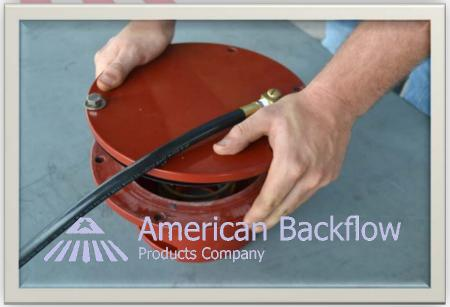
Replace seat disc on the back of the housing.
