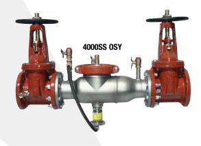
Series 4000SS Reduced Pressure Zone Assemblies are designed to provide protection of the potable water supply in accordance with national codes. This series can be used where approved by the local authority having jurisdiction on health-hazard cross-connections. Series 4000SS features short lay length, lightweight stainless steel body, corrosive resistant stainless steel relief valve, and patented cam-check assembly.
