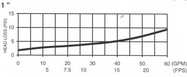
FLOW RATE (GPM) VELOCITY (FPS)
