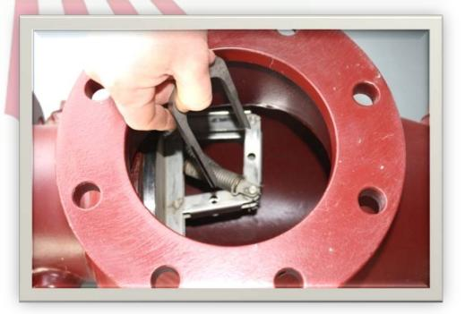
Push retainer clip into the linkage holes on the knuckle joint.
