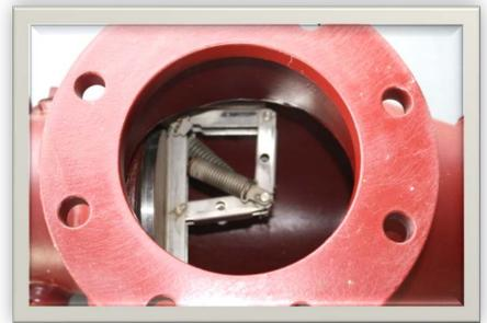
Check valves are knuckle joint assemblies that are **side mounted**.
