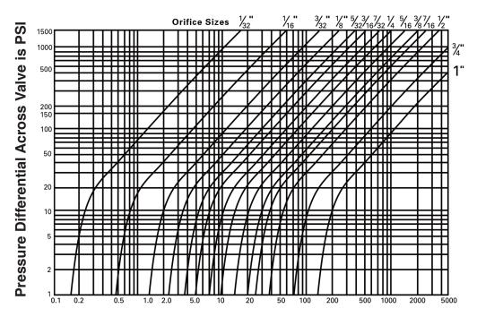
**Venting Capacity in Cubic Feet of Free Air Per Minute**
