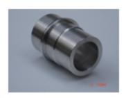
The Flow Nozzle is sandwiched between the 2-1/2" supply hose and the FlowBuster's female swivel fitting to allow higher accuracy readings for smaller flow conditions (100-750 GPM). The Nozzle Insert is available in two sizes, 1-1/8" and 1-3/4".
