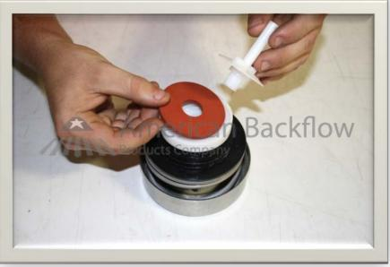
With lower guide removed, place the module upside down on a clean surface.
