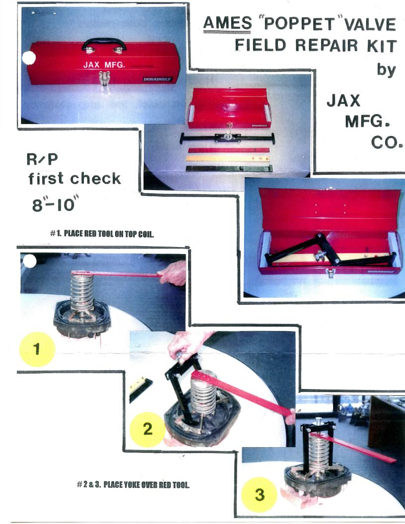
using wrench tighten until the spring compresses to free the disc from the body of the check
