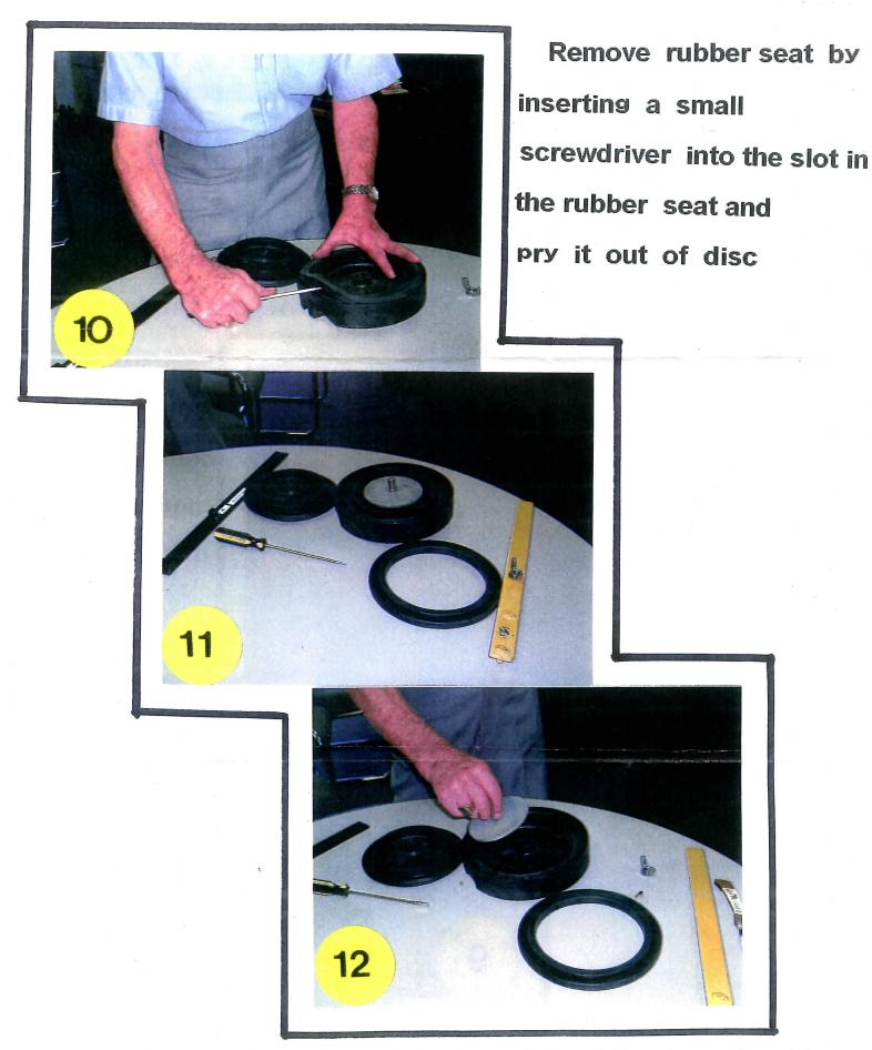
Seat can now be replaced Insert new seat rubber and reassemble in reverse order
