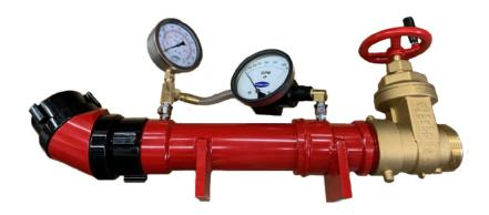
Accurately measures outlet static and residual water pressures and flow from 2 ½" hose connections. The "Enforcer" facilitates the initial and periodic testing of pressure regulating valves in sprinkler and standpipe systems per NFPA 13, NFPA 14, and NFPA 25 requirements. This versatile device can also be used for standpipe, fire pump, and hydrant flow testing.
